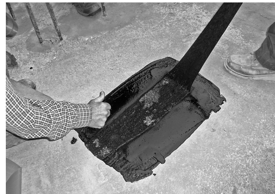
Figure Y – Cohesive failure (pass)
